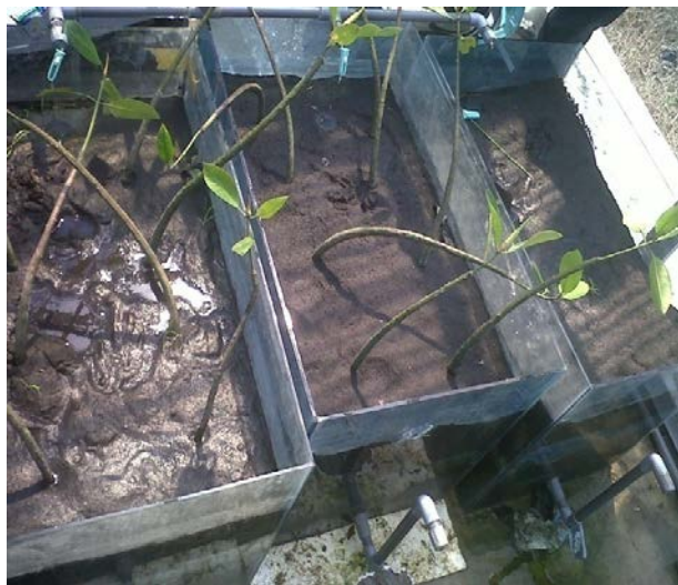
Gambar 5 Subsurface Flow Wetland
