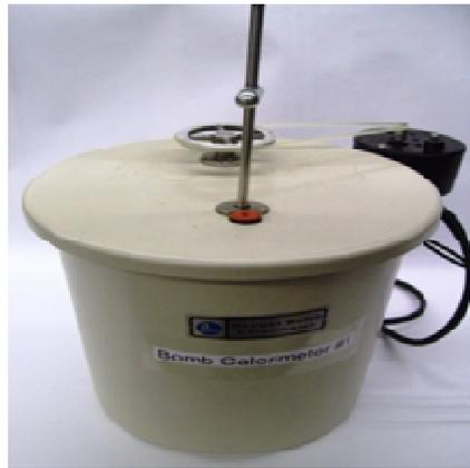
Gambar 1. Kalorimeter Bomb
