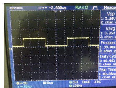
Gambar. 10. Tampilan Osiloskop pulsa PWM 40 kHz
