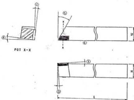
Gambar 4. Geometri pahat bubut Semented Carbide (SC)
