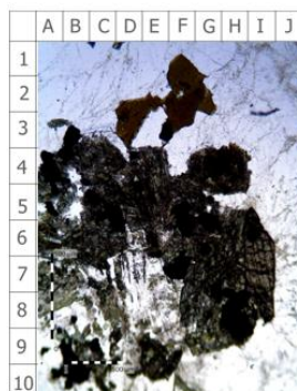
Fig. 7. Granite existence in a petrography on the example of Sices 1.L5. Captured by microscope polasisari magnification 40x.
