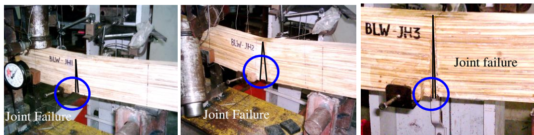
Figure 6. The pattern damage of BLW-JH
