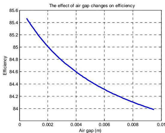
Figure 6. Efficiency with Respect to the Air Gap
