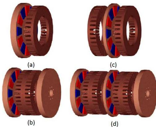
**Figure 1. Axial Flux Machine Configurations. (A) Single Rotor-Single Stator Structure, (B) Two Rotor-Single Stator Structure, (C) Single Rotor-Two Stator Structure, (D) Three Rotor - Two Stator Structure**
