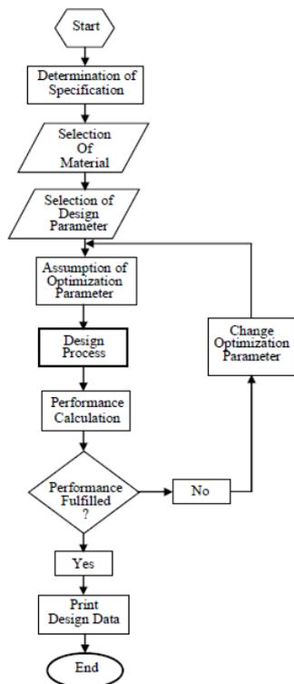
Figure 3. Flow Chart of the Design Process
