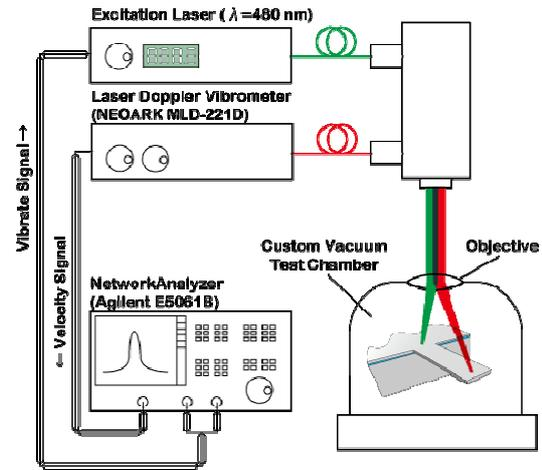
Fig. 3. The Measurement System of the Cantilever
