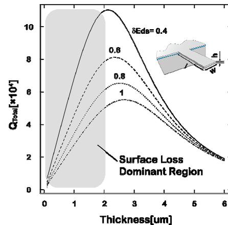
Fig. 2. The Theoretical Curve of  $Q_{Total}$  as a Function of its Thickness. The Length and Width are 150 $\mu m$  and 30  $\mu m$  with the Cantilever, Respectively.  $\delta E_{ds}$  is a Parameter Related to Surface Energy Loss
