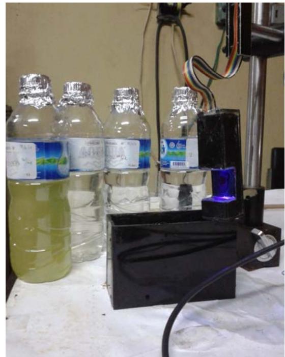
Figure 2. Optical Probe and Measurement Container
