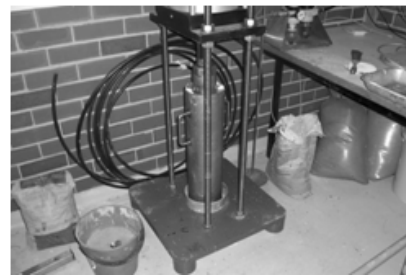
Figure 5. Consolidation of kaolin slurry in cylindrical mould
