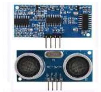
**Gambar 2.** Sensor Ultrasonic HC SR-04
