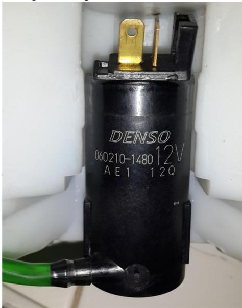
Gambar 2. Pompa Air Wiper
