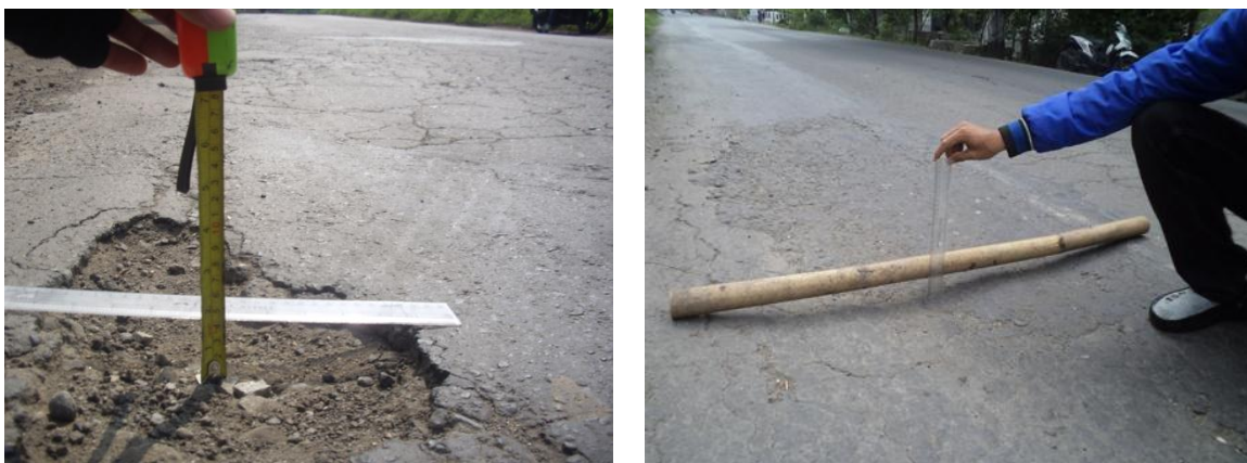
Figure 4 Sample Road Condition Survey
