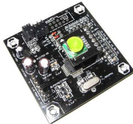
Gambar 5. DT-Sense Barometric Pressure and Temperature Sensor [6]
