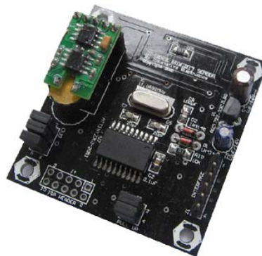
Gambar 4. DT-Sense Humidity Sensor [1]
