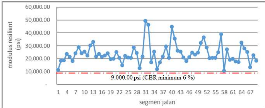
Gambar 4 Modulus Resilient Tanah Dasar Ruas Nomor 017.11(K) Jalan Bypass Demak Arah Kudus
