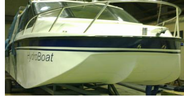
Gambar 5. Surface Effect Planing Hull (SEP-Hull)
