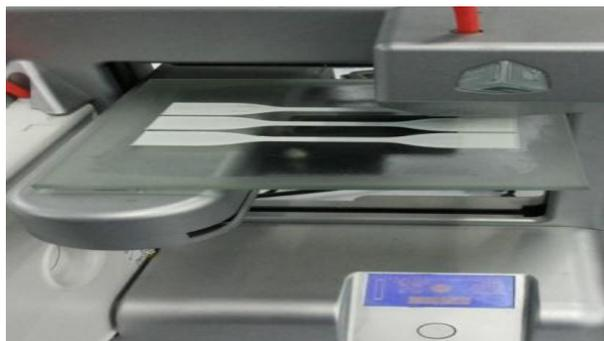
**Gambar 10.** Proses *3D Printing* Orientasi Horizontal Bahan PLA
