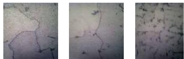
Gambar 6. Struktur Mikro dari the Undeformed (a), the Deformed (b), dan the Unfailed Blade (c), pembesaran 500X
