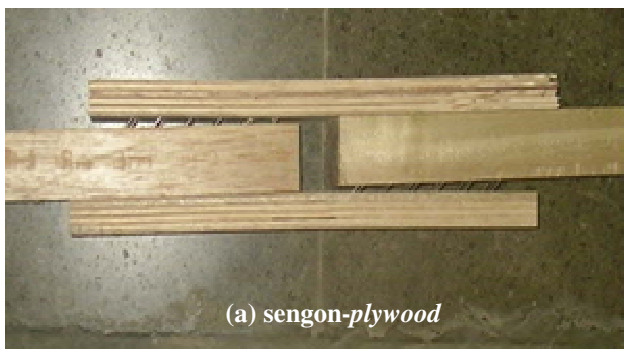
Figure 11. Failure at three rows - six nails tension specimen (a) sengon -plywood (b) meranti -plywood
