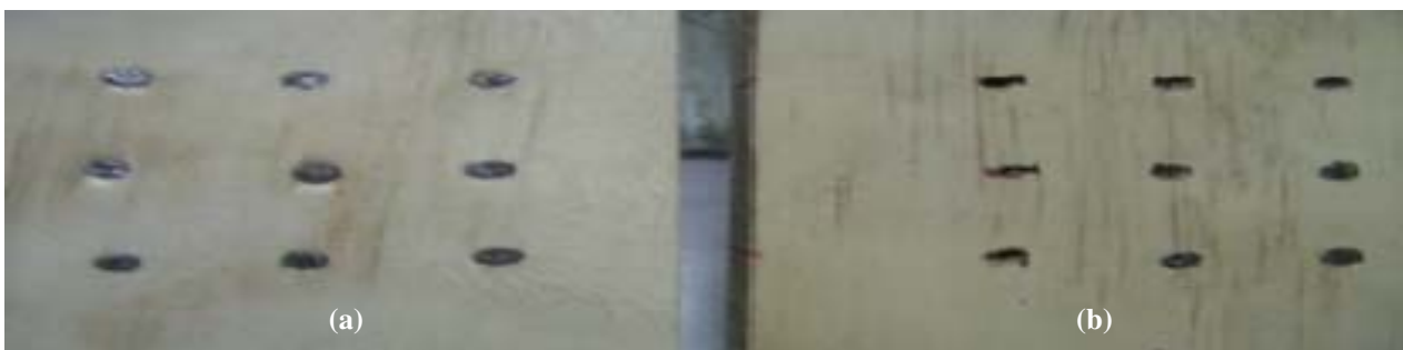
Figure 13. Damage on the outside surface of plywood sides plate, (a) sengon -plywood (b) meranti -plywood
