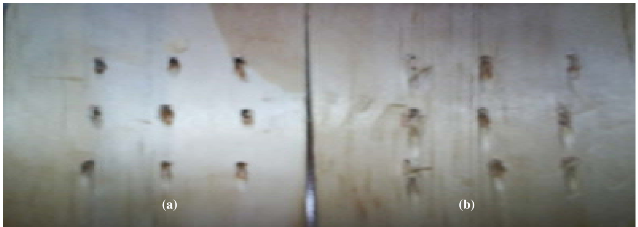
Figure 14. Damage on the inside surface of plywood sides plate, (a) sengon -plywood (b) meranti -plywood
