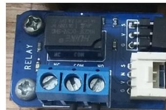
Gambar 6 Contoh gambar relay
