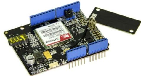
Gambar 6 Rangkaian GPRS Quadband Shield V2.0
