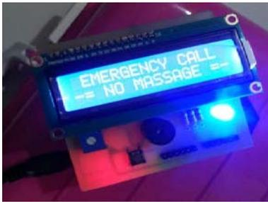
Gambar 16 LCD disaat GPRS Off
