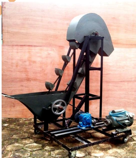
Gambar 2. Prototipe *bucket elevator*
