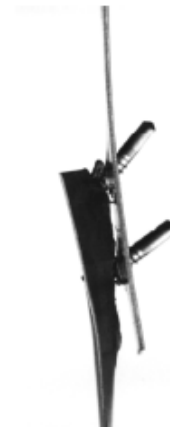
Gambar 9 Keruntuhan Tilting & Pull-Over [Dunai et all, 2004].
