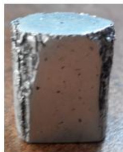
(b) Feed rate 0.459; Cutting speed 320 Rpm; Depth of cut 0.5 mm.
