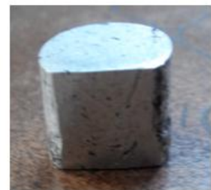
(c) Feed rate 0.459; Cutting speed 850 Rpm; Depth of cut 0.5 mm.
