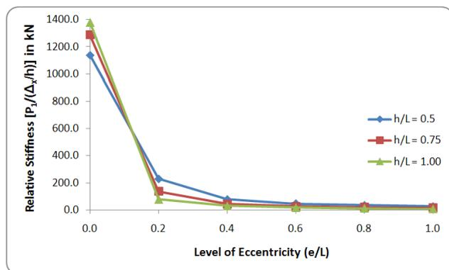
Figure 6. Relation between Level of Eccentricity and Relative Stiffness of EBFs (Thene 2009)
