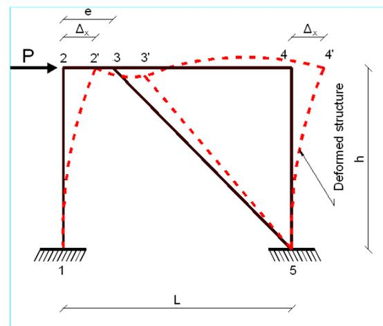
Figure 2. An EBF under Lateral Loading
