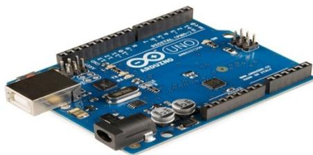
Gambar .1. Board Arduino
