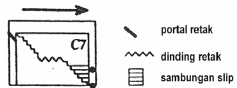
C Diagonal crack
