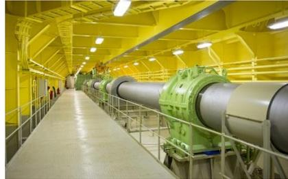
Gambar 1. *Propeller Shaft* [2].
