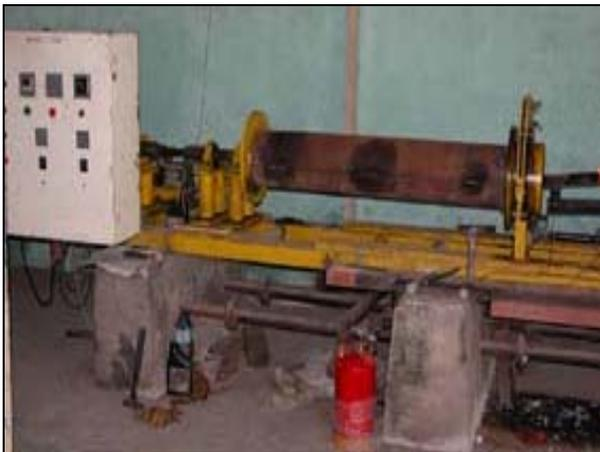
Gambar 4. Mesin Centrifugal Casting
