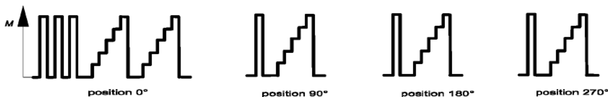
Gambar 2 Langkah pengambilan data kalibrasi torsi static.
