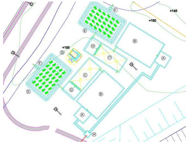
Gambar 3 Layout Instalasi Pengolahan Lindi
