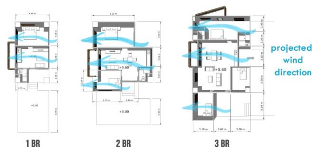
Figure 7. The Internal Room Planning Arrangement
