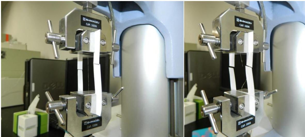
Figure 3. Tensile test of Abaca fiber before test (left) and after test (right)
