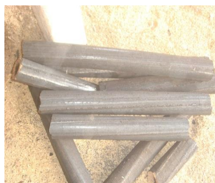
Fig. 2 Coir dust and rice husk blend briquettes at mixing ratio of 50:50
