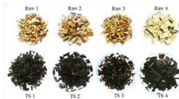
**Fig. 4** Physical appearances of raw and torrefied biomass
