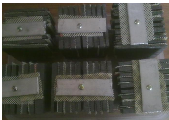
Fig. 2 Grid structure of biomass battery
