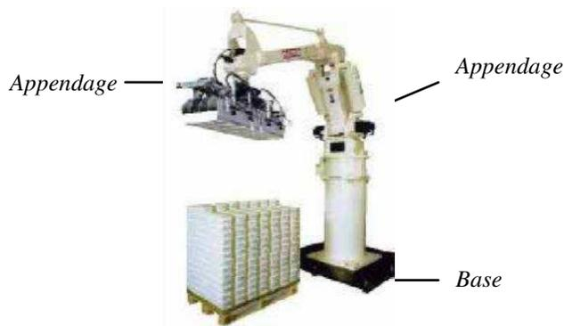
Gambar 1. Robot manipulator [3].
