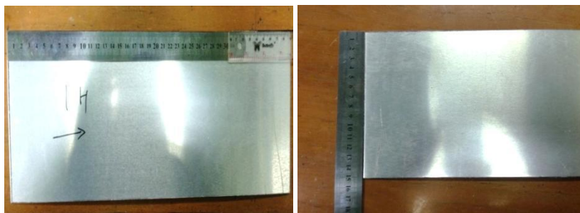
Gambar 2. Material AA 60661-O 300 x 150 mm
