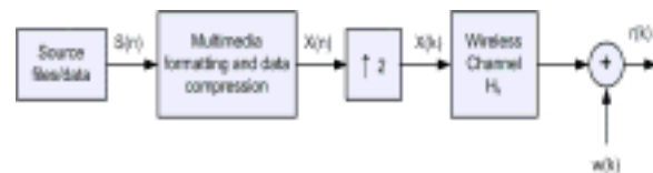
Figure 2. Transmitter block for T/2 baseband communication system
