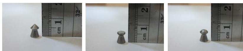
Gambar 2. Conical Nose, Flat Nose, Hemispherical Nose
