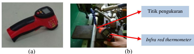
Gambar 6. (a) Infra red thermometer , dan (b) proses pengukuran temperatur pahat.
