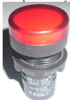
Gambar 8. Lampu indikator inverter.
