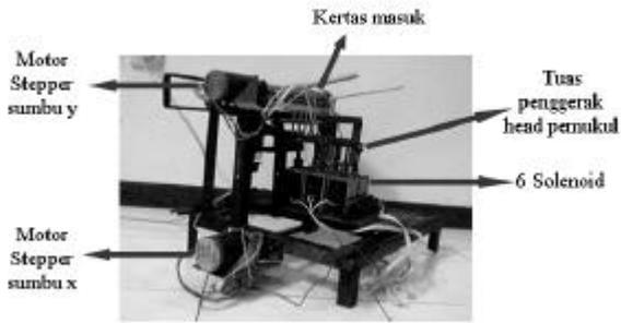
Gambar 8. Model Mekanik Mesin Printer Huruf Braille
