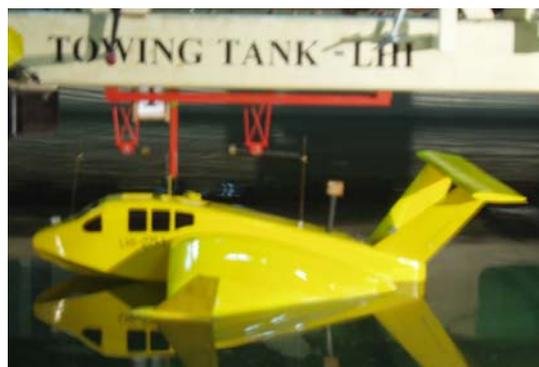
Gambar 3. Pengujian *Captive Test* model *WiSE Craft*
