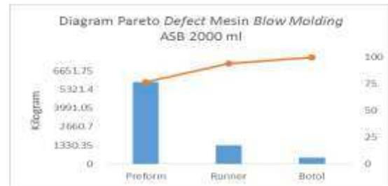
**Gambar 6** Diagram Pareto Defect Mesin Blow Molding ASB 2000 ml
