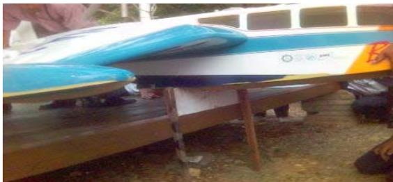
**Gambar 2.4.1.3** Pengukuran *Weight and Balance*, dudukan di sekitar *center of gravity, c.g.*
