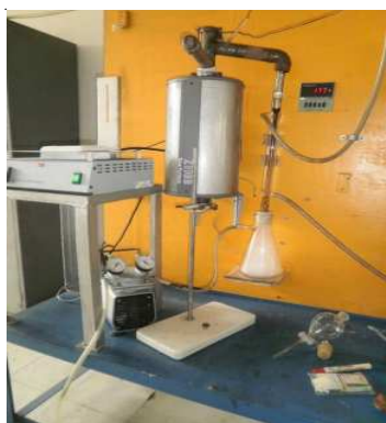
Gambar 2. Rekayasa alat pirolisis ( Lab Scale )
