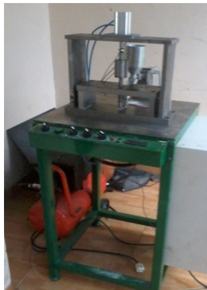
Gambar 1. Hasil rancang bangun mesin pencetak bulir SRG Figure 1. SRG forming machine prototype
