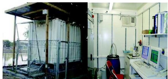
Gambar 1 Stasiun Pemantau Kualitas Air Sungai otomatis MERMAID (Marine, Environmental Remote-Controlled Monitoring and Integrated Detection) di sungai Surabaya
