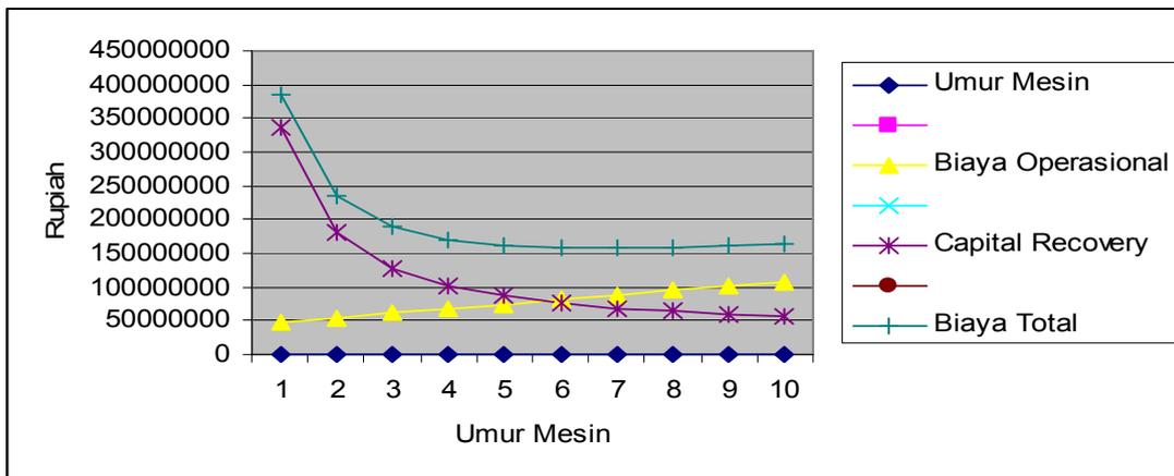
Gambar 3. Umur Ekonomis Mesin Moulding I
